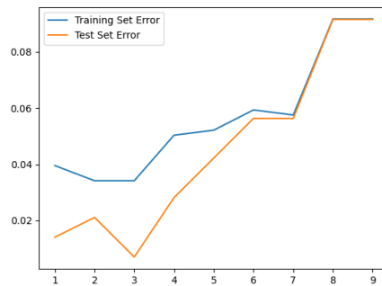
Figure 3: The testing and training error rate plotted against the number of random features ( m ) for each weak learner
