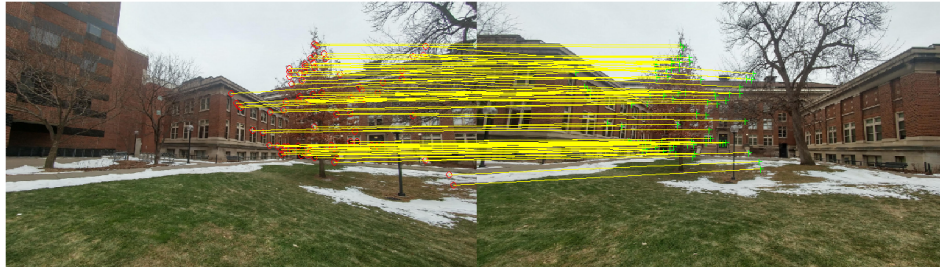
Figure 4: You will compute a homography using SIFT matches filtered by RANSAC.
