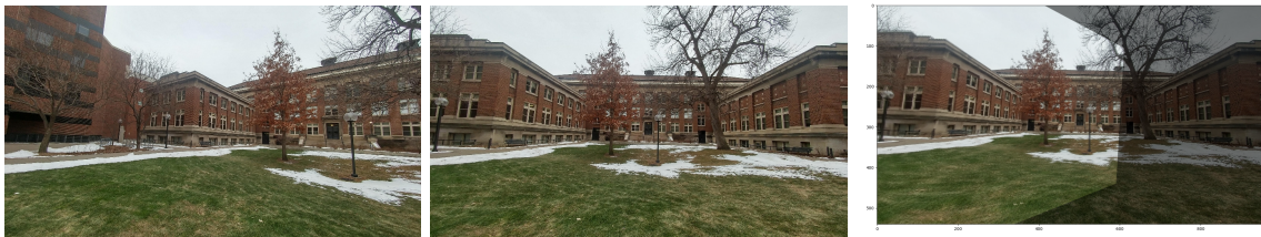
Figure 2: Results of homography matching. The left image is warped to appear from the same perspective as the middle image.
