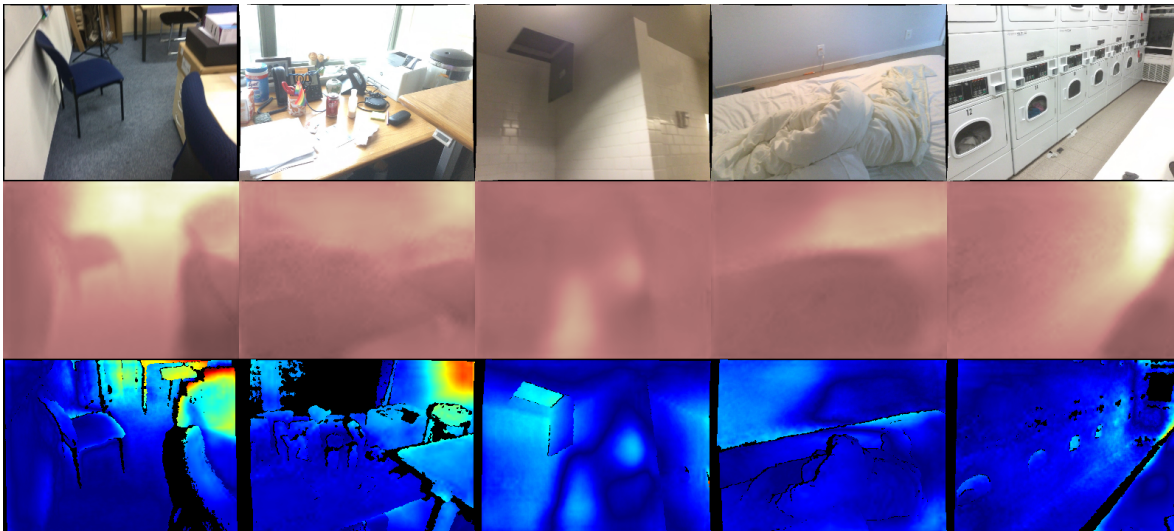
Figure 3: Depth maps' error visualization. Top: images; Middle: predicted depth maps from an ExtendedDepthNet ; Bottom: predicted depth maps' error (the colder color indicates the smaller error).
