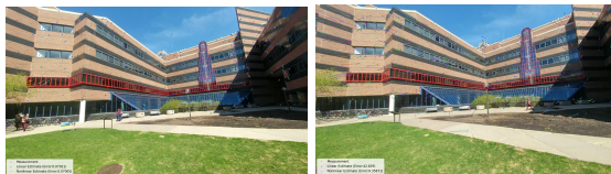
Figure 5: Results of the bundle adjustment step. The top figure shows a typical case where the reprojection error goes from 0.079 to 0.070. The bottom image shows a case where there was large error due to PnP_RANSAC and Triangulation. Bundle Adjustment fixed the incorrect points and decreased the error from 42.6 to 0.359.
