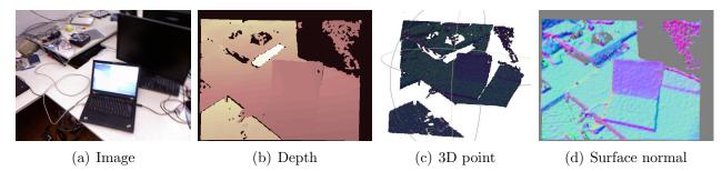
Figure 2: Given a depth image (b), you will generate 3D points and surface normal using inverse projection.
