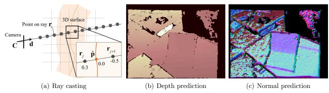
Figure 5: Given a TSDF and camera pose, you will predict the 3D points and surface normals using ray casting.
