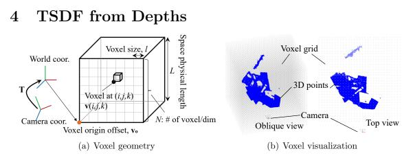
Figure 3: Given a depth image (b), you will generate 3D points and surface normal using inverse projection.
