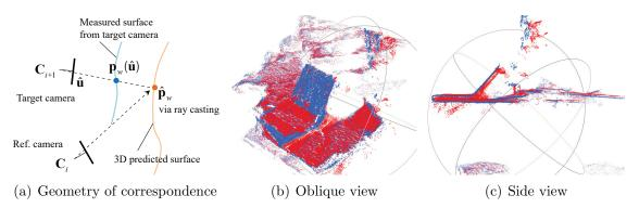
Figure 6: Correspondence between the predicted (red) and measured (blue) points are visualized.
