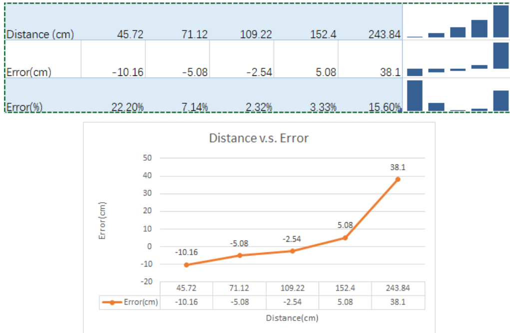
Figure 7. Distance vs. error curve of our robot’s attempts of hitting five targets of increasing distance.
