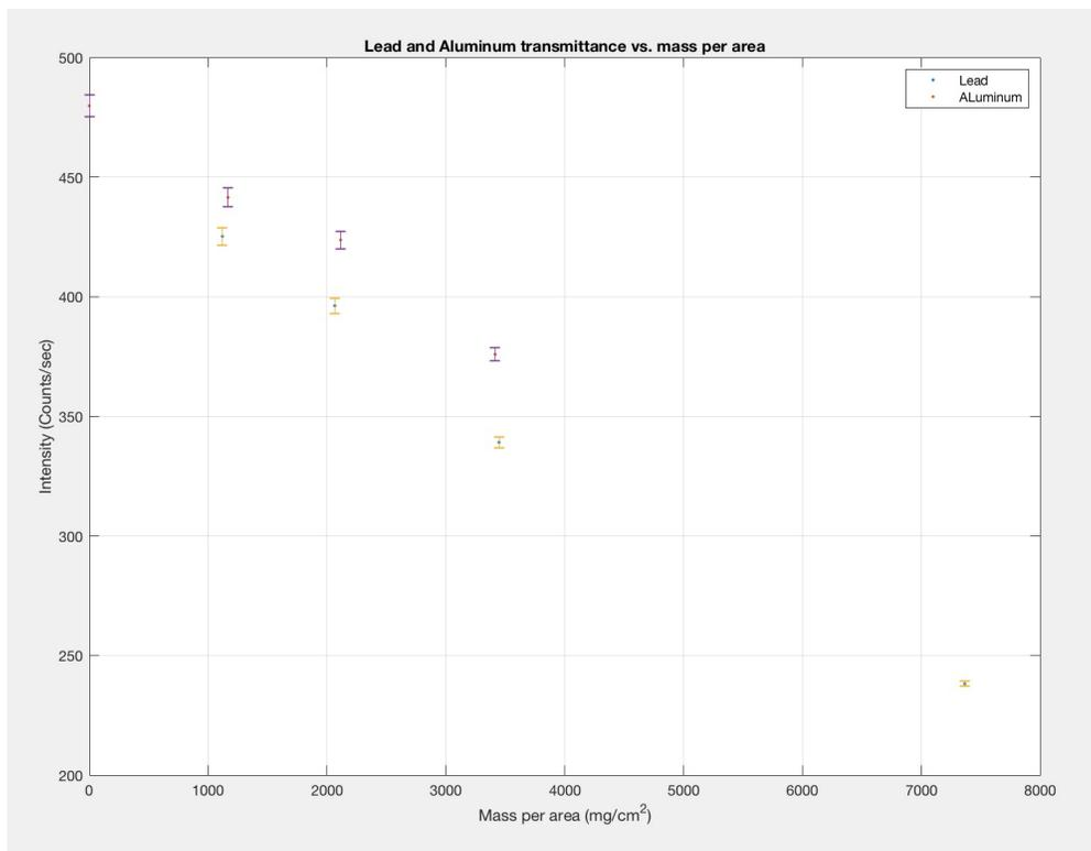
Figure 2: Our measured intensity vs. mass per area for Lead and Aluminum
