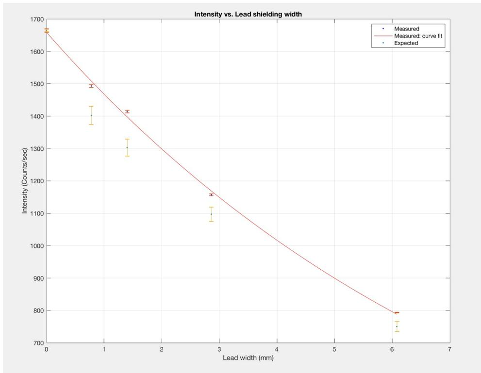
Figure 1: Our measured intensity vs. thickness for the lead barriers
