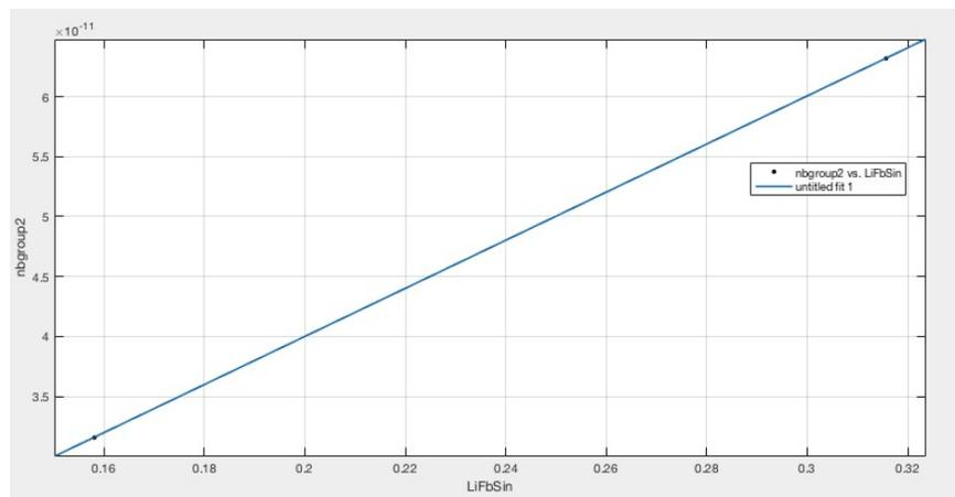
Figure 7: LiF  $n\lambda/2$  vs.  $\sin(\theta)$  for  $K_\beta$
