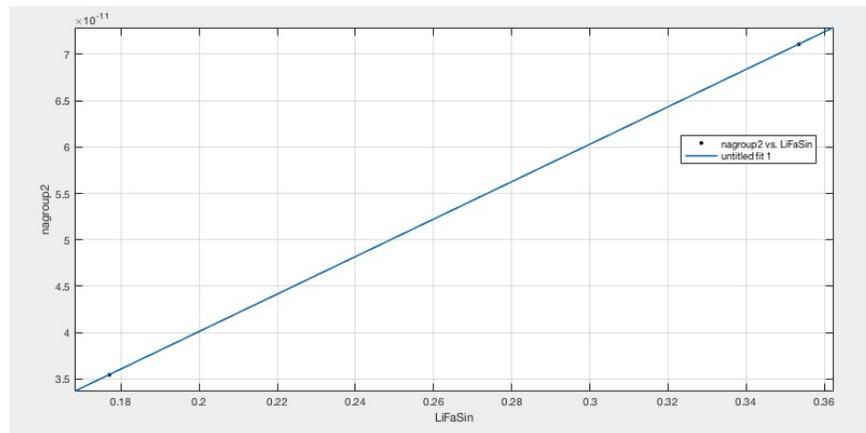
Figure 6: LiF  $n\lambda/2$  vs.  $\sin(\theta)$  for  $K_\alpha$
