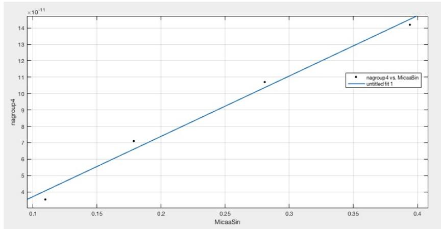
Figure 12: Mica  $n\lambda/2$  vs.  $\sin(\theta)$  for  $K_\alpha$
