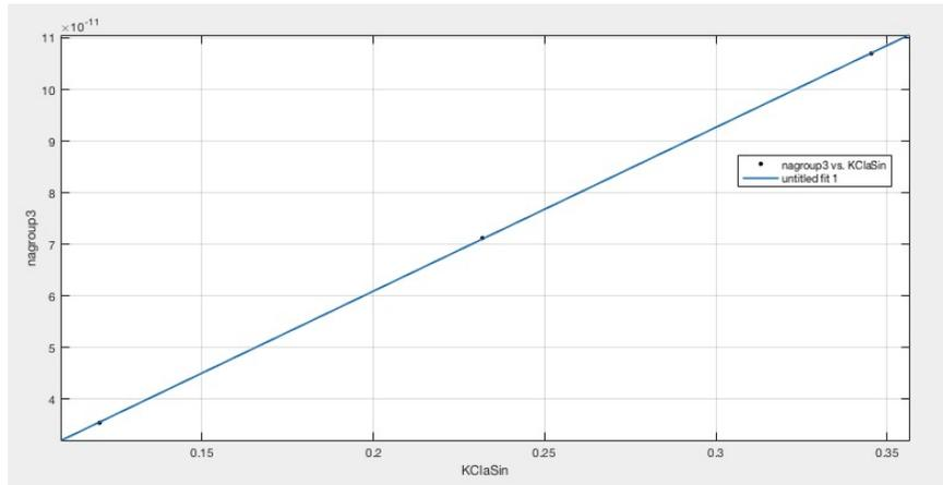
Figure 10: KCl  $n\lambda/2$  vs.  $\sin(\theta)$  for  $K_\alpha$
